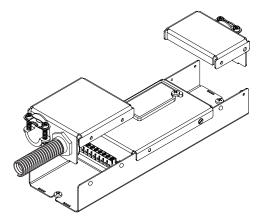
4) Snap covers in position and secure with provided fasteners.
