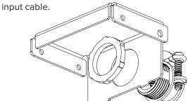
3) Thread cables through conduit/strain reliefs and covers; then make connections as required.
