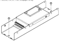
2) Terminal covers support 1/2" strain relief of conduit. Conduit or armoured cable must be used on power input cable.
